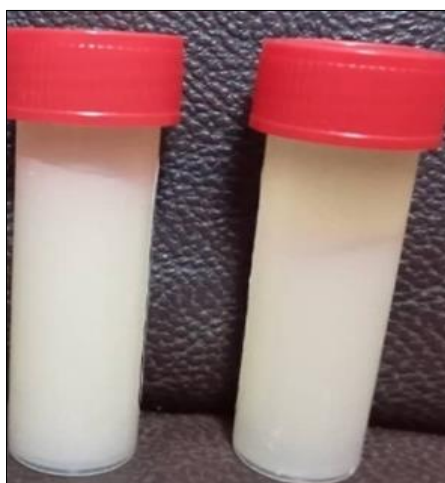
Figure 4 Samples F5 and F1 showing varying degree of phase separation after centrifugation at 4000 rpm for 10 min over two cycles
