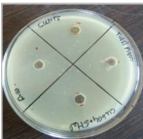
Figure 2 Antibacterial activity of copper nanoparticles (Cu-NPs) against Bacillus subtilis as evaluated by the agar well diffusion method
