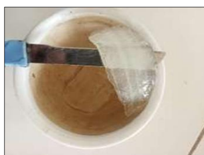
Figure 9 Placing the Gel into Mortar to Homogenize it
