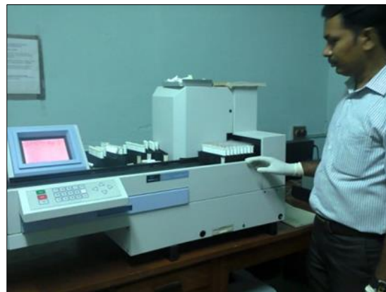
Figure 4 Melatonin Assay by RIA counted in a gamma counter from Automatic Gamma Counter (Perkin Elmer=Tri-Carb 2910 TR), Perkin Elmer, USA
