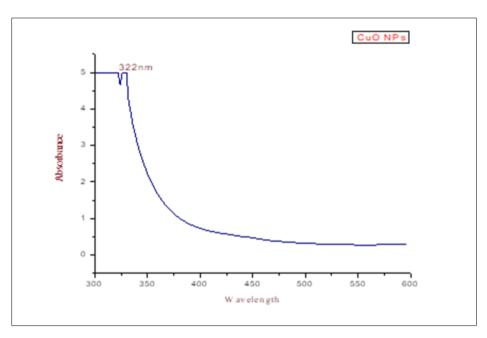
Figure 1 UV-Visible Spectroscopic image of CuO nanoparticles
