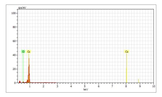
Figure 3 Energy Dispersive X-ray Spectroscopic (EDAX) image of CuO nanoparticles
