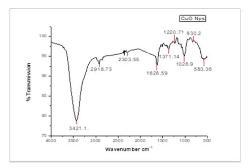
Figure 4 Fourier Transform Infrared Spectroscopic image of CuO nanoparticles
