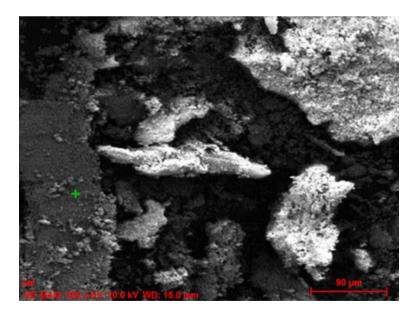
Figure 2 Scanning Electron Microscopic image of CuO nanoparticles
