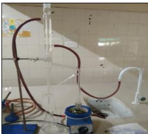
Figure 1 Extraction of essential oil by Clevenger apparatus
